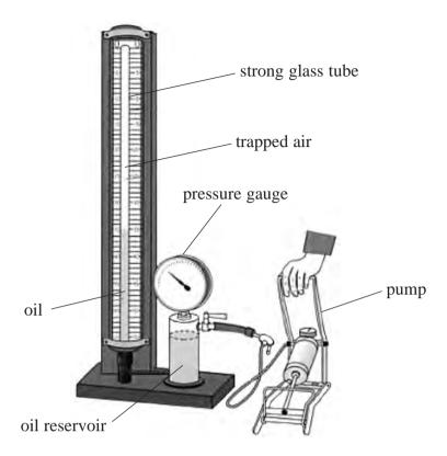
Air is trapped in a glass tube of uniform cross-sectional area. As the pressure of the trapped air is increased, the length of trapped air decreases. The student collects data and plots the following graph.
